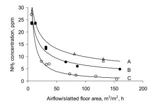
**Figure 13.** Ammonia concentrations according to airflow rate when the air is exhausted with a fan in the wall (A), exhausted through a separate exhaust air duct (B), and exhausted through the manure channel (C) in a house for growing-finishing pigs.
