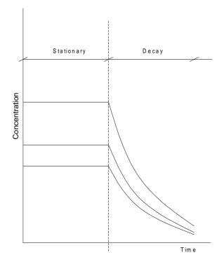
Figure 3. Example of tracer gas concentrations during a trial.
