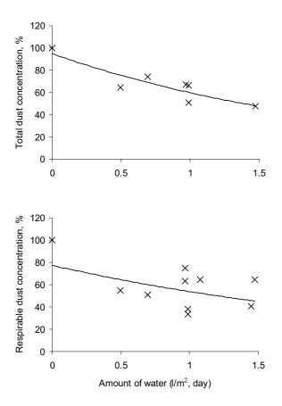
Figure 9. Relative levels of dust concentrations when flat fan nozzles were used (reference level is 100%).
