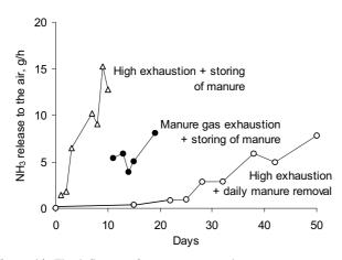
Figure 14. The influence of manure storage time on conveyors on ammonia release in an aviary system for laying hens when ventilation air is exhausted at roof level (high exhaustion) and when the air is exhausted through an air duct close to manure conveyors (manure gas exhaustion).
