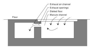
Figure 4. Two investigated principles for manure gas exhaustion.
