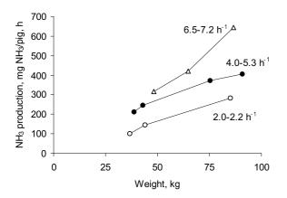
Figure 12. Release of ammonia in a house for 64 growing-finishing pigs in relation to pig weight and air exchange rate after 24 hours manure storage.
