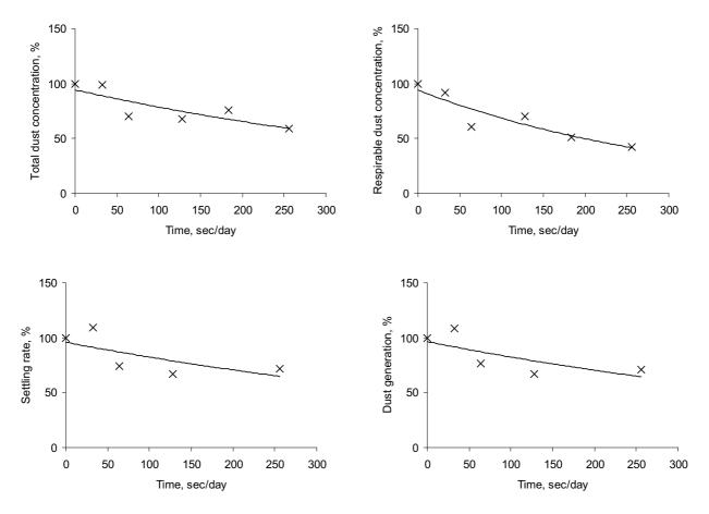
Figure 10. Influence of humidification on total and respirable dust concentrations, settling rate and generation of dust as a function of the spraying period when full cone nozzles were used (reference level is 100%).
