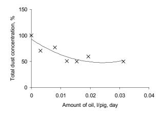
Figure 11. Relative changes in dust concentration when an automatic oil spraying system has been used.
