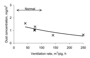
**Figure 8.** The influence of ventilation rate on total dust concentration in a building for growing-finishing pigs with an average body weight of 67.0 kg.
