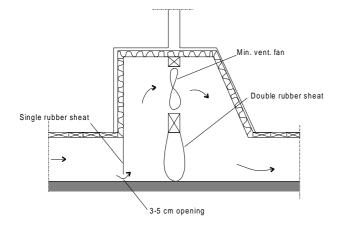
Figure 1. Methods of preventing gas leakage into the building when manure is handled in the liquid or solid state.
