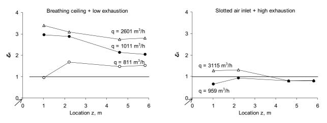
Figure 15. Ventilation effectiveness ( $\varepsilon_x$ ) at different distances from the injection point of an air pollutant (z, m) at two combinations of air inlets and air outlets. The pollutant is released at the arrow. q = ventilation rate, m<sup>3</sup>/h.
