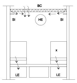
Figure 2. Design of the calf stable where tracer gas measurements took place. HE – high exhaustion; LE – low exhaustion; BC – breathing ceiling; SI – slotted inlet; x – measuring place.
